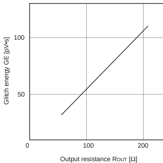
Fig. 2. Output resistance vs. Glitch energy
