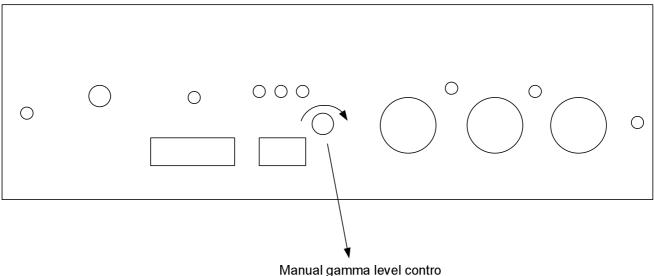
We can see the panel between Switch and component input, there is a little screw, it is use for gamma level adjust. Below is adjustment way:
