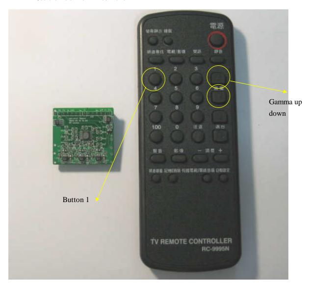
Button 1: input select (switch on the card should set to hdmi side first),
