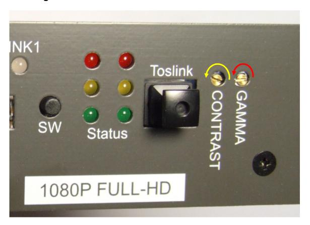
We can see the panel, there is two little screw, one for contrast adjustment (need professional person to do this), another one use for gamma level adjustment. Below is adjustment way:
