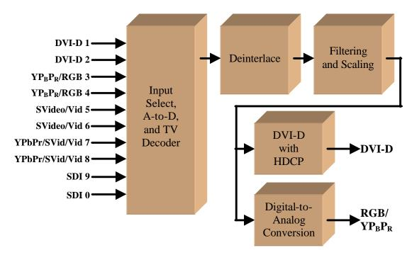
VisionPro HDP Functional Block Diagram
