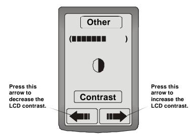
Figure 4-15: Adjusting the contrast
