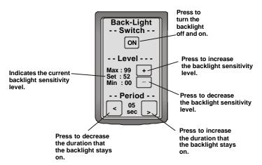
Figure 4-16: Adjusting the backlight
