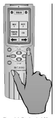
Figure 2-2: Turning the LCD on
