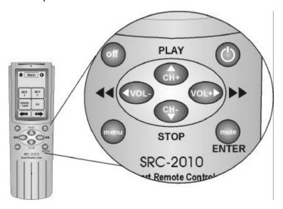
Figure 2-4: Direct access buttons
