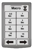
Press one of the listed durations (0.5 seconds to 15 seconds) if you want to have a time delay occur between device commands.
