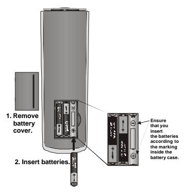
Figure 2-1: Inserting the batteries
