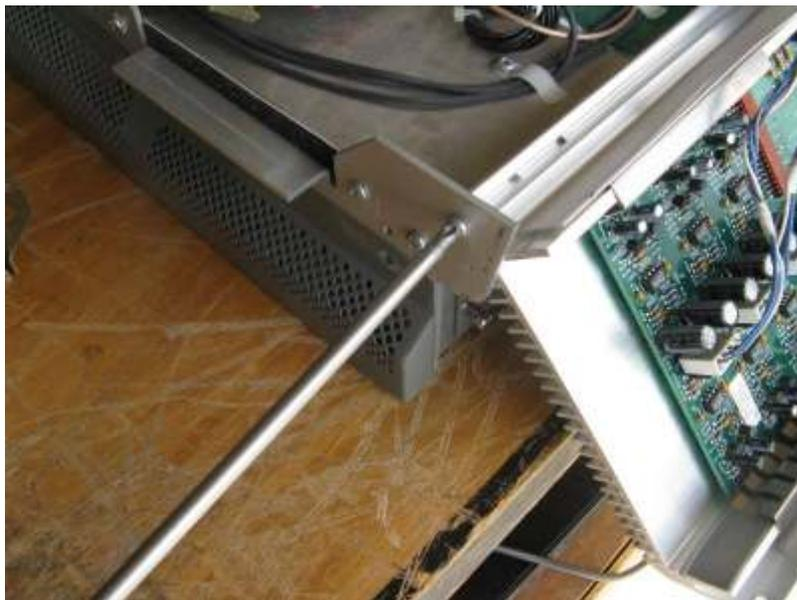
12) Now it's time to remove the Focus and HDM. It will help to remove the lead shielding to do this and it's a good idea anyway. I suggest some Windex and paper towels to clean off as much of the Black sooty deposits as possible. This stuff is very conductive and will encourage high voltage arcing in a set.
