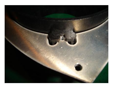
Insert the provided nylon spacer between the aluminum adapter plate and the plastic lens mount flange. Thread the #6 stainless steel screw through the aluminum plate, the nylon spacer, and finally into the nut and tighten. Repeat 4 times for each lens.
