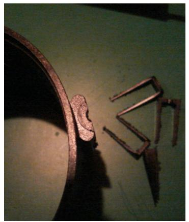
Cut notches where the old screw holes existed. They should be just wide enough to clear the shafts of the #6 screw provided. If you cut two slots on either side you should be able to easily break out the middle piece.
